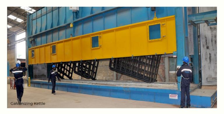
Dorman Long recently commissioned Zinco International to perform an ultrasonic inspection on our Hot-Dip Galvanizing Kettle to provide an impression of kettle walls and its condition after its years in service. The result from this inspection prompted our decision to replace the kettle. This is a maiden project, planned and executed for the first time with a planned schedule of 36 calendar days which started from 1st September 2022 concluding on 6th October 2022.
